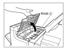
2 Lift knob ① (See the upper right figure), then remove any misfed paper.
